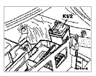
Battery voltage is continuously supplied to terminal 30. A 10 A fuse is installed between terminal 30 and 30a. The fault memory is continuously supplied with voltage via terminal 30a. When the ignition is switched on, the relays are controlled by electronics via terminal 15. In this way the ABS (N30) and 4MATIC (N30/3) control units are supplied with voltage via terminal 87E and additional equipment via terminal 87L.
