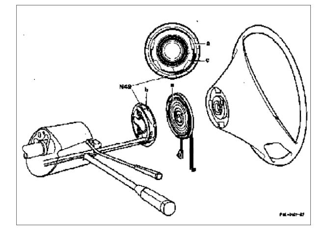
N49 Steering angle sensor a Plastic slip ring
