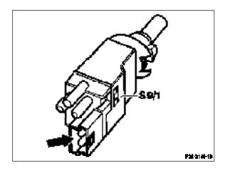
When the service brake is operated, the 4MATIC control unit (N30/3) receives a signal via a cable (d) whereby the 4MATIC is switched off. The second cable de-energizes the ABS control unit (N30).
